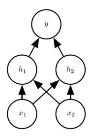
"Rectified linear activation": out =  $max(0, W^{T*}x+c)+b$
