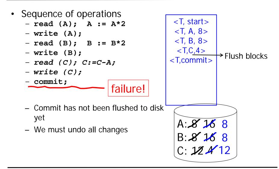
Sequence of operations <T, start> - read (A); A := A\*2<T, A, 8> - write (A); <T, B, 8> - read (B); B := B\*2 <T,C,4> - write (B);  $\rightarrow$  Flush blocks <T,commit> - read (C); C:=C-A; ►Flush log - write (C); - commit; failure! No problem, TX has finished normally A: 8 16 Nothing to do, all committed B: **8** 16 changes are on disk C: 1/2 4
