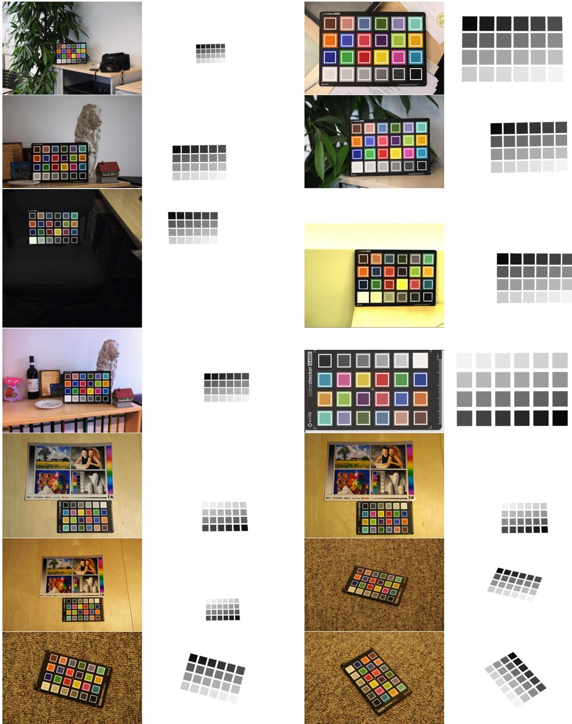
Figure 23: Shown are all images used in the evaluation with their respective reference image next to them. The inner of the white quadrilaterals shows the computed area used for color extraction.
