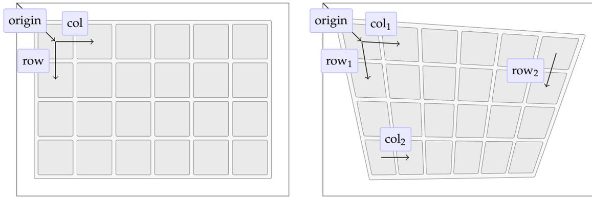
(a) The patches of the color chart are addressable using an affine coordinate system using only integer coordinates. (b) In the image the affine coordinate system becomes a bilinear coordinate system. Please note that four vectors would suffice to describe the transform instead of the displayed five (for example by replacing  $row_2$  and  $col_2$  with their sum  $row_2 + col_2$ ).
