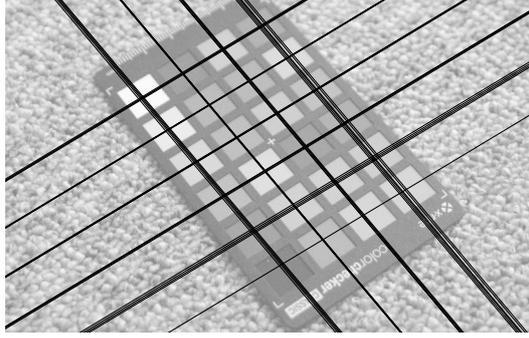
(a) Shown are crosses through every region center with both cross lines being parallel to the axes of the intermediate coordinate system. Clustering is clearly visible which allows to assign row and column numbers to each region.
