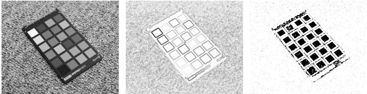
(a) The *ProcessingImage* resulting (among other things) from color averaging the original input image (*FullImage*). (b) The *GradientMagnitude* of the *ProcessingImage*. Dark regions have non-zero gradient magnitude. (c) Image (*Homogeneous*) of the pixels considered 'flat' (dark color).
