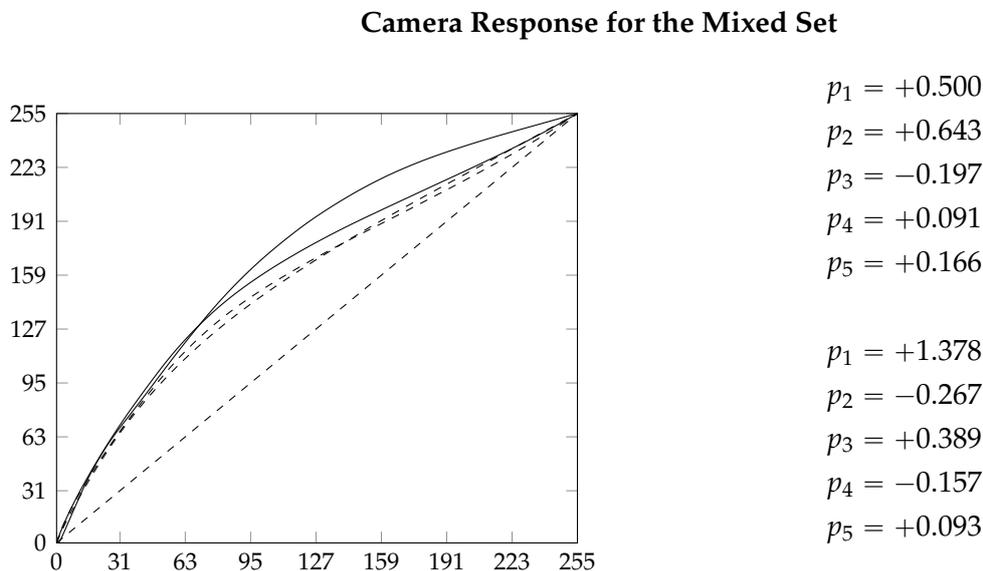
Figure 19: The calculated response curves for the mixed set and the factors for the base functions  $h_1$  to  $h_5$ . The dashed lines show the responses calculates in the single camera scenarios.
