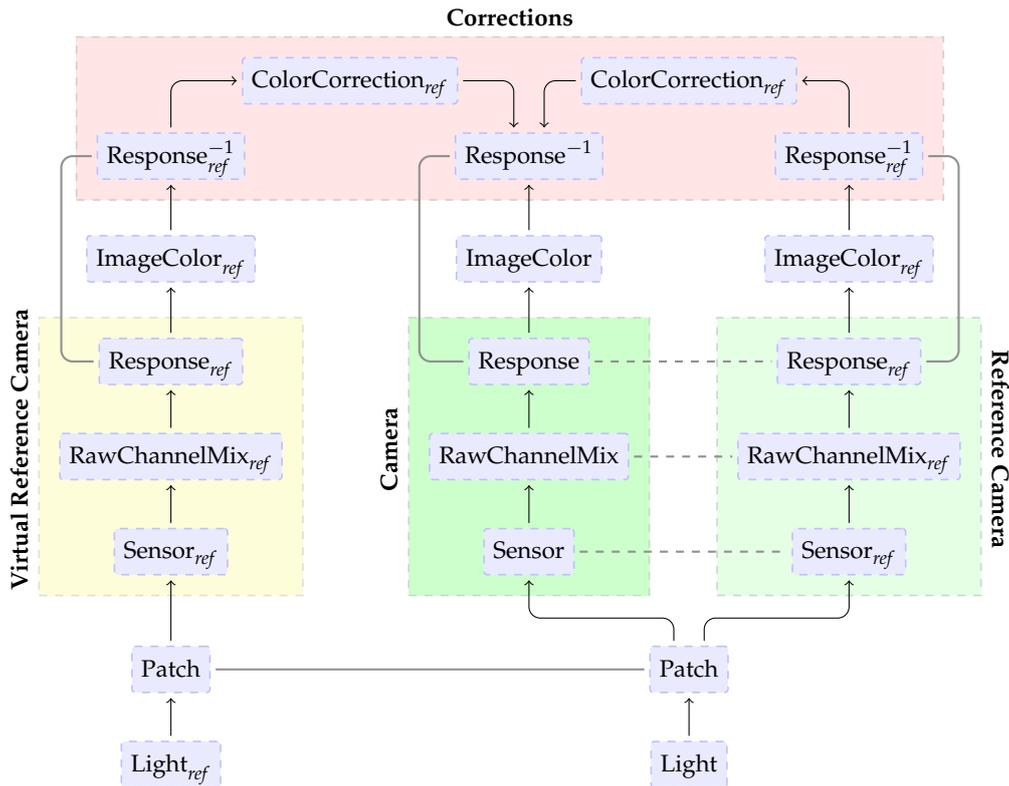
Figure 9: Shown are the functions involved in ‘creating’ and correcting image colors. Parameters, which ideally would be equal, but most likely won’t, are joined by dashed lines and parameters, which assumed or intended to be equal, are joined by solid lines.
