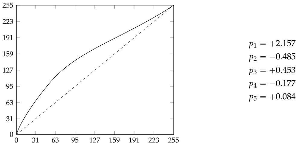
Figure 15: The calculated response curves for the EOS 400D series and the factors for the base functions  $h_1$  to  $h_5$ .
