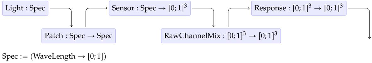
Figure 8: A general camera color model in form of chain of functions.
