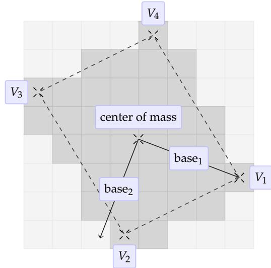
Figure 3: Finding the vertices of a rasterized quadrilateral.
