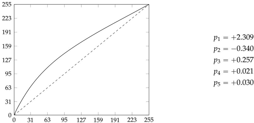
Figure 18: The calculated response curves for the PowerShot A650 series and the factors for the base functions  $h_1$  to  $h_5$ .
