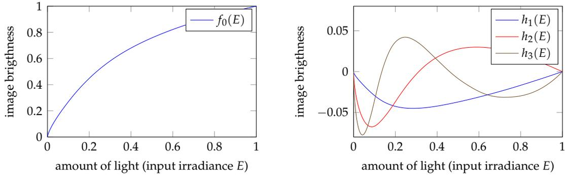
(a) The first base vector which is the average of all camera response functions used to calculate the principal component analysis. (b) The further base functions of the vector space of response functions. Please note the smaller vertical scaling.
