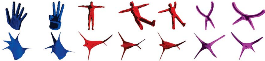
Figure (1.2): Spectral embeddings of articulated shapes. The coordinates of the spectral embeddings are given by the (eigenvalue normalized) eigenvectors corresponding to the lowest non-zero eigenvalues.
