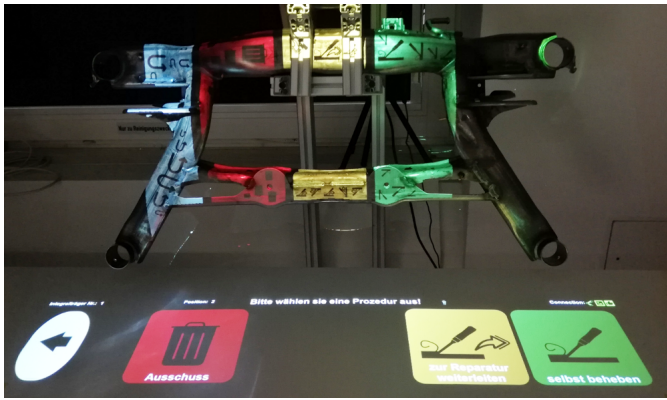
Fig. 2. Example application of projection mapping in an industrial scenario. The menu structure on the table is duplicated on the surface of the workpiece. By using the projection distortion-based tracking the projection can be used for object tracking.
