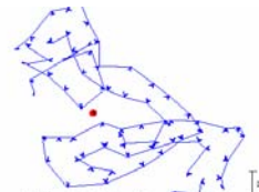
(b) Map estimate derived by treating odometry measurements as if they were exact.
