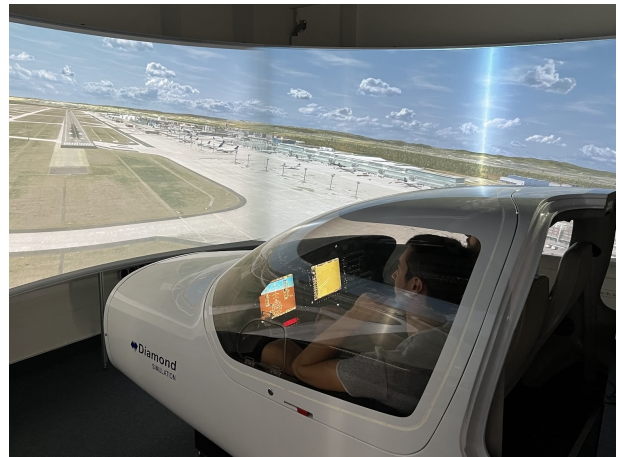
(b) Pilots were flying in a full-size Diamond DA40 aircraft flight simulator. The cockpit resembles the full functionality of a real cockpit.
