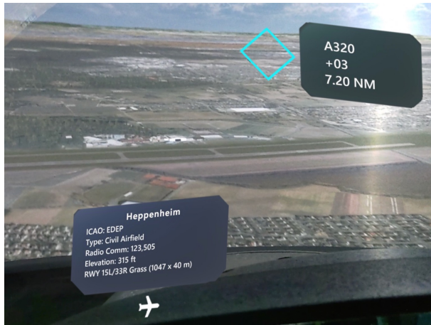
(a) Exemplary virtual components displayed by the prototype to accompany an aircraft (upper right) and an airport (lower left) in the vicinity.
