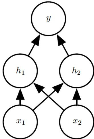
“Rectified linear activation”:  $\text{out} = \max(0, W^T \cdot x + c) + b$
