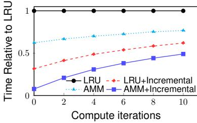
**Fig. 16: Relative completion time (processing cost)**
