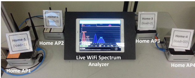
Fig. 5. Demonstrator Setup consisting of four home APs and a real-time spectrum analyzer showing the current channel allocation.
