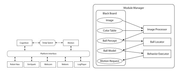
Fig. 1. Schematical illustration of the platform interface (left) and the module architecture (right).
